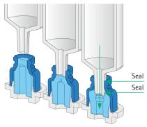
The safe-flow valve is exposed, making it easy to disinfect. The needle-free valve opens upon connection and automatically closes upon disconnection, thus allowing fluids to be drawn overhead without difficulty.
